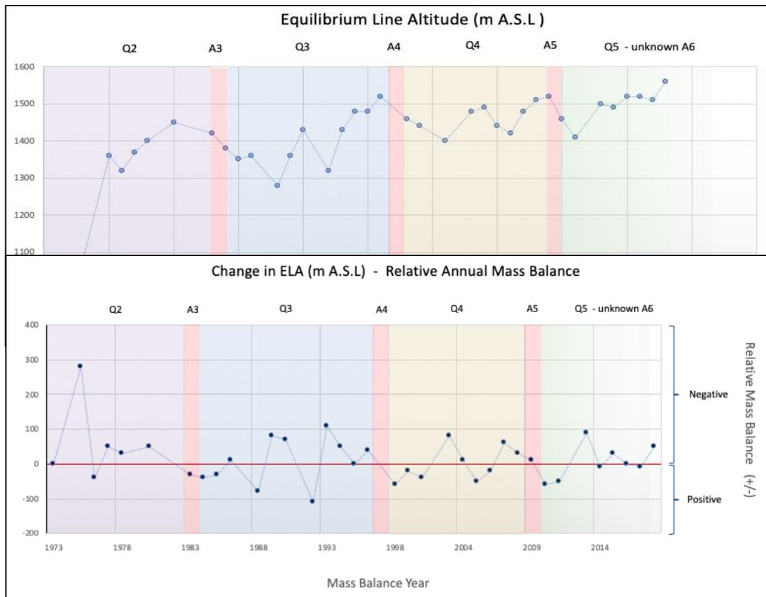
**Fig. 3.** ELA timeseries (1973-2018): ELA derived from snowline at the end of the balance year (late August – early September) using satellite imagery. Surge events derived from Bevington and Copland (2014); categorized into quiescent and active phases.
