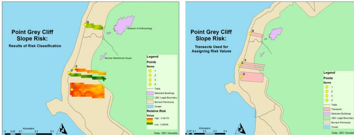
**Fig. 6.** Point Grey Cliff Risk Classification of Slope: Normalized slope angle from UBC LiDAR (left), transects used for sites 1 – 4 (right).
