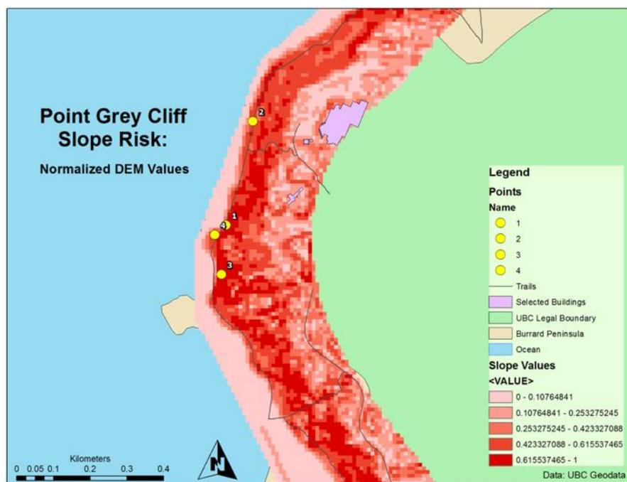
**Fig. 5.** Risk classification based on slope angle of our study area. Slope values are normalized 0-1 from a 0-90° classification of a 10 x 10 meter resolution DEM derived from UBC LiDAR data.
